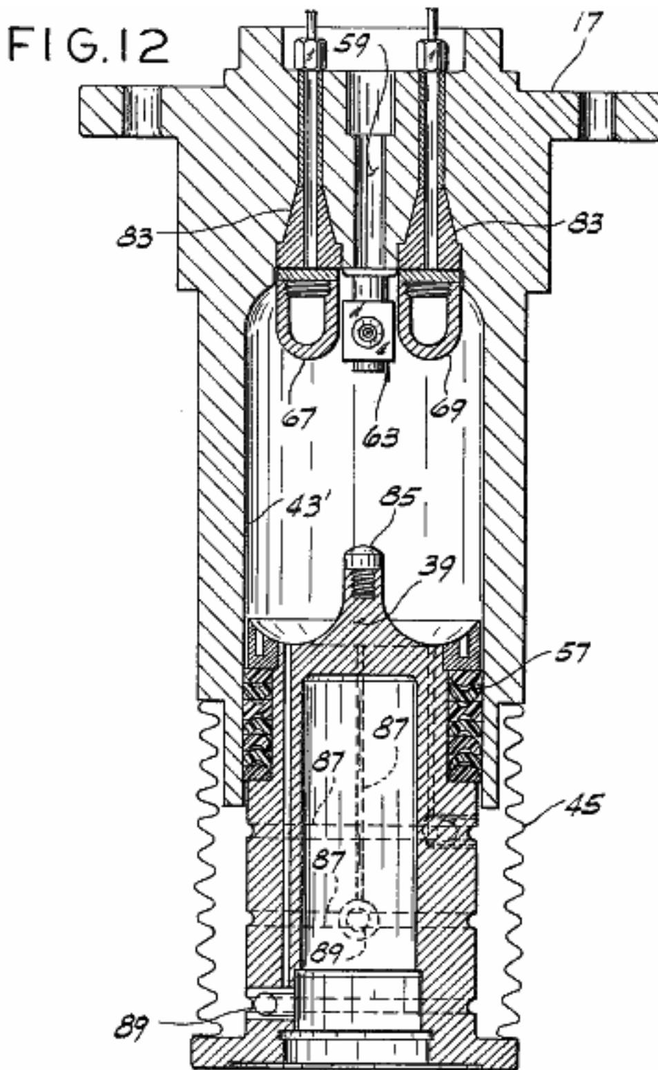
Fig.12A is a cross-sectional view similar to Fig.5 and Fig.12, but on a reduced scale and with parts broken away, showing an additional embodiment of a cylinder head used in an engine of this invention:
