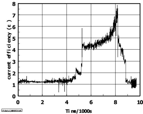
Fig. 4C: Change of current efficiency ( $\epsilon$ ).
