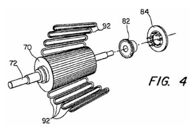
Fig.4 is an exploded perspective view of the basic components of the motor of Fig.3.
