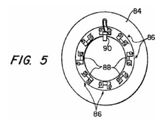
As shown in **Fig.5**, the brush holder **84** includes eight brush mounts **86**, each of which defines a slot **88** in which a pair of brushes is mounted. One brush **90** is shown in **Fig.5**, it being understood that two such brushes are mounted in each slot **88** so that sixteen brushes are required.
