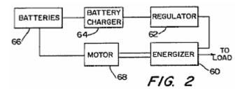
Fig.2 is a block diagram of the overall energy-producing system of the invention
