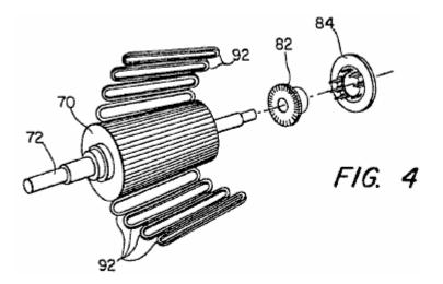
A commutator **82** is also mounted on shaft **72**, and co-operates with associated brushes (not shown in **Fig.1**), to conduct current to the windings of armature **70**. This co-operation is shown best in **Fig.4** which is an exploded view, illustrating the armature **70**, commutator **82** and a brush holder **84**.
