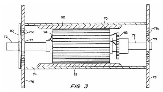
Fig.3 is a partially sectioned side elevational view of a modified electrical motor constructed in accordance with the invention.
