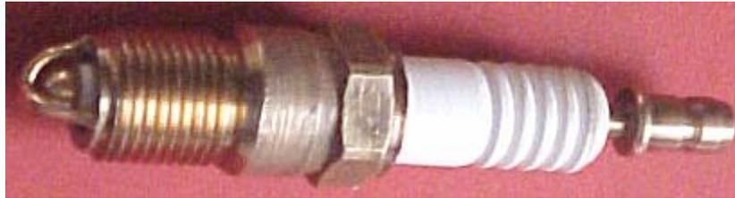
However, this plug is far from ordinary. The central electrode has been changed from a cylindrical post to a hemispherical dome, surrounded by four arched electrodes, each of which being positioned at a constant distance from the hemisphere. This allows a much greater spark area and results in very much improved performance.
