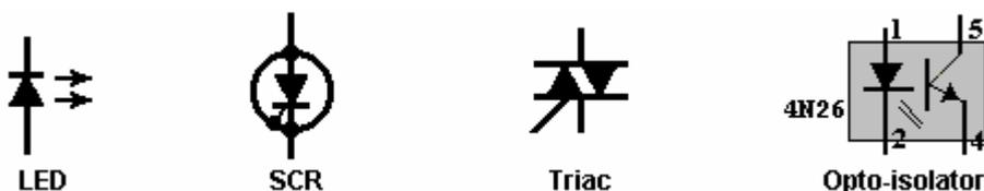
**LEDs:** There is a widely used variation of the diode which is extremely useful, and that is the Light Emitting Diode or 'LED'. This is a diode which emits light when carrying current. They are available in red, green, blue, yellow or white light versions. Some versions can display more than one colour of light if current is fed through their different electrical connections.
